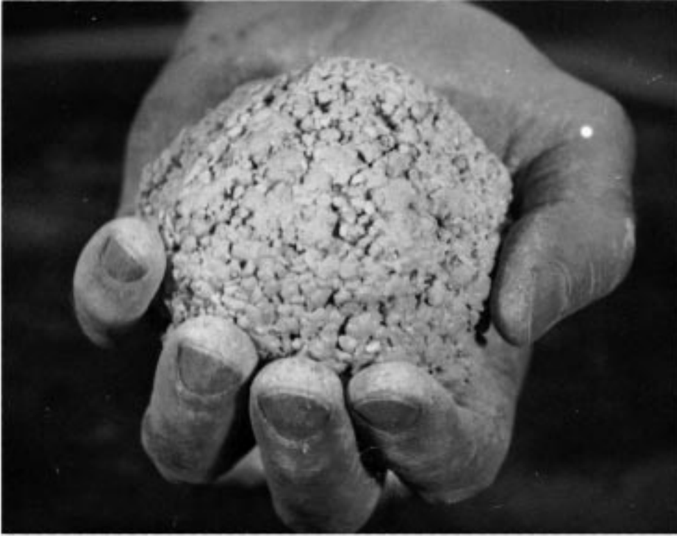
FIG. 3 Range in Consistency of Castable Mixes as Shown by Ball-in-Hand Tests
